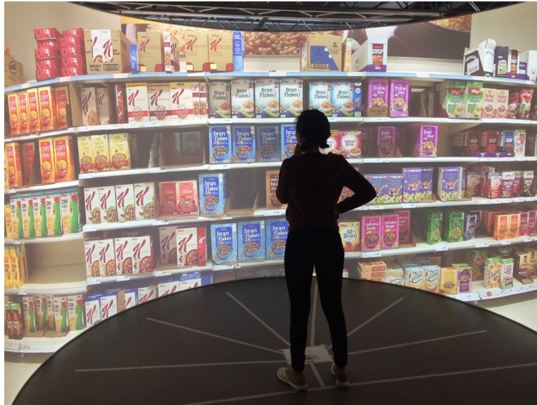
Figure 2. High resolution photograph of supermarket shelves projected on 200°-degree wrap-around screen
