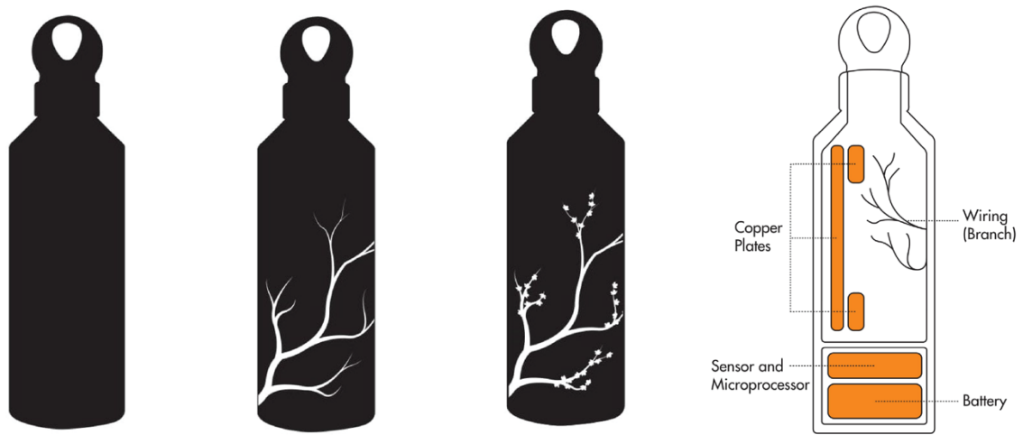
Figure 2: States of the bottle and technical details
