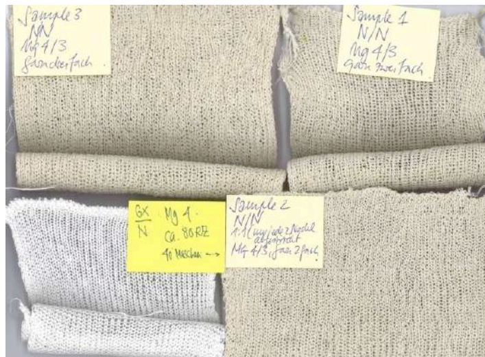
Figure 16. Knitted patterns with rotor yarn Nm 10. Source: Lucerne School of Art and Design.
