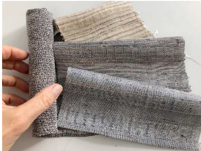
Figure 20. Woven samples with silk warp and banana weft. Source: Lucerne School of Art and Design.
