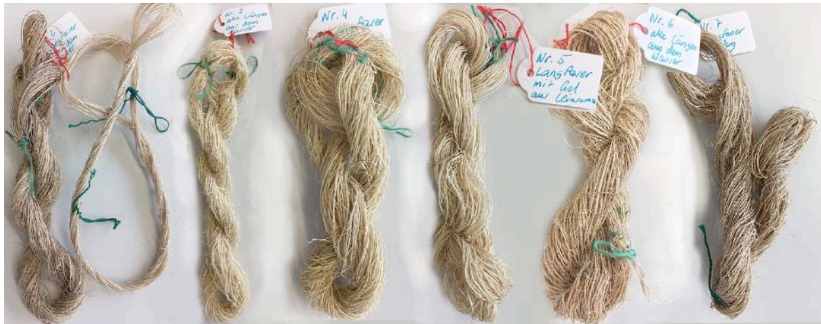
Figure 9. Handspun yarn from banana fibres. Source: Lucerne School of Art and Design.
