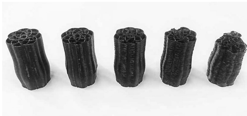
Figure 2. Chasen handles, 3D printed at different speeds (from left to right - 1,2,3,4,6 times the standard speed of the 3D printer)
